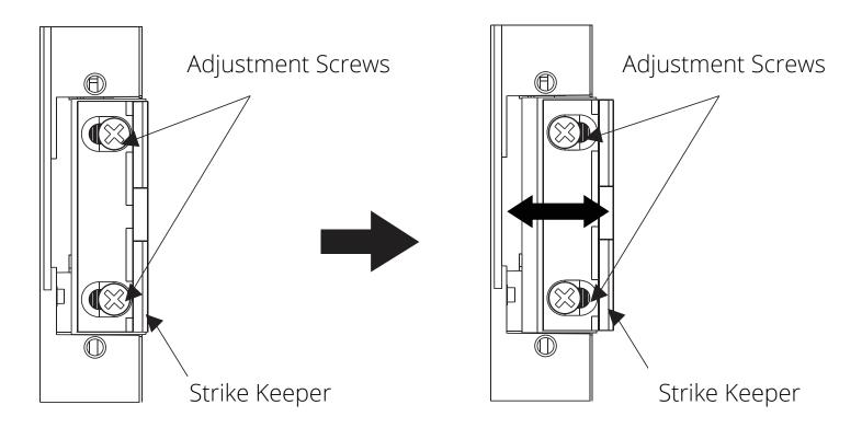
The strike keeper can be adjusted up to a maximum of 3 mm to easen the installation on doors that may be warped. To adjust, simply loosen the indicated screws and adjust the protector to the required distance. The strike keeper allows the latch to open and close without the need to make or drill additional holes in the door.
