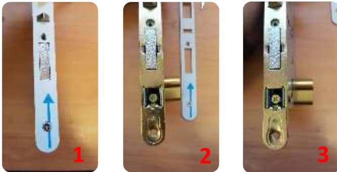
A After fitting the lock body in the door thickness, remove the frontal plate and screw the cylinder using the screw supplied.
