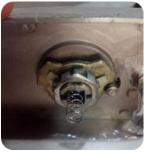
Insert springs inside each handle in order to fix the lever in the right position.
