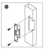
Mount the lock and connect the power to perform a test.
