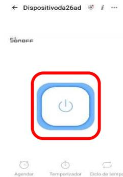
By pressing the symbol the device will manually activate or deactivate. This function can also be achieved by pressing the button on the device.
