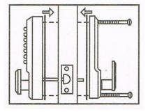
Before final tightening, check that the lock is in a vertical position and that the mechanism operates freely.
