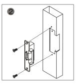
Assemble the lock and turn on the power to test.
