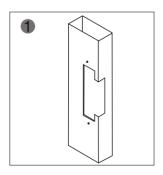
Cut hole according to the size of the latch.
