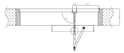
Loosen the four clamping screws to adjust the length of the push arm according to the depth "L" of the door frame, make the angle between the push arm and the door leaf is 90° as shown in the diagram below.
