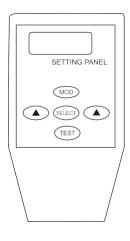
Connect the configuration panel to the door controller and adjust the parameters:
