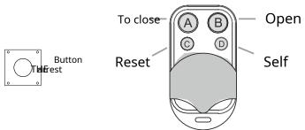
Instructions for code matching between remote control and drive unit controller: 1. Delete: Long press the "Code" button until the buzzer sound stops, release the button.
