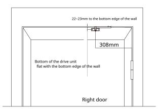
The push arm fixing seat is fixed to the door leaf with two round-head wood screws according to the size shown in the diagram. (If it is a steel door, fix the fixing seat with M6x15 cross screws).
