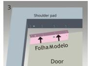
Mark on the door and shoulder the location of the screws in the fitting plate;
