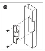
Mount the latch and connect to the power supply to perform a test.
