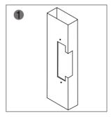
Cut the hole according to the latch size.
