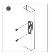
Fix the electric latch in place.
