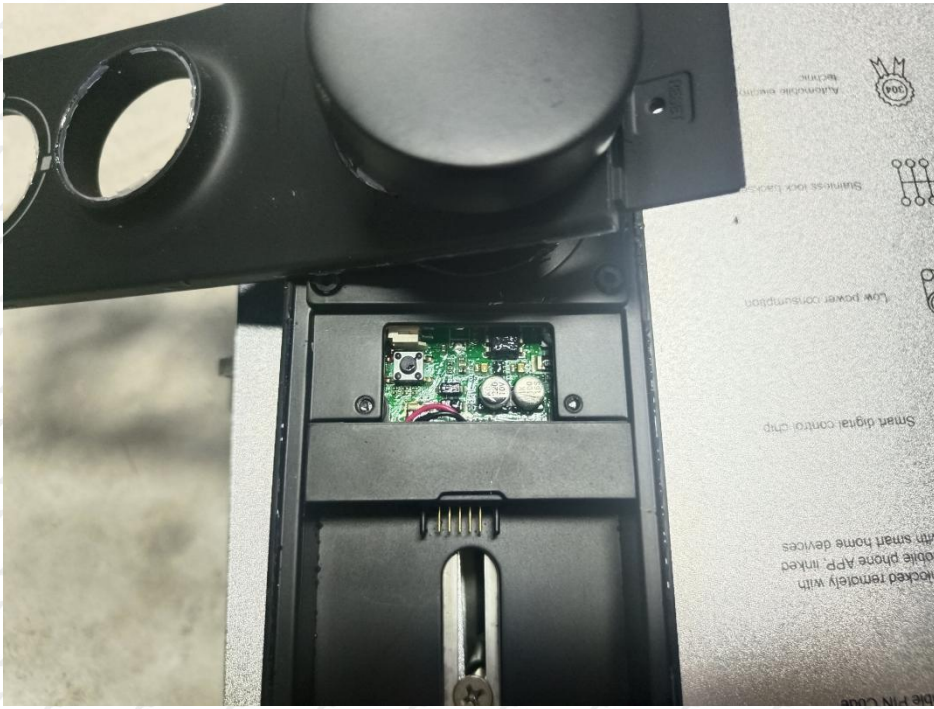
Photo 3: (internal) After dust test
