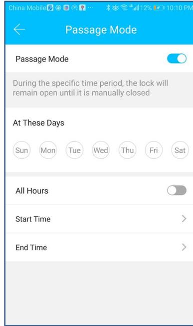
In the main interface of the app, select the passage mode in the settings, and the date of the passage mode can be set, and the start time and end time of the passage mode can also be set. After the passage mode is activated, everyone can directly unlock the door without any access permission. The passage mode can be turned off by clicking again.
