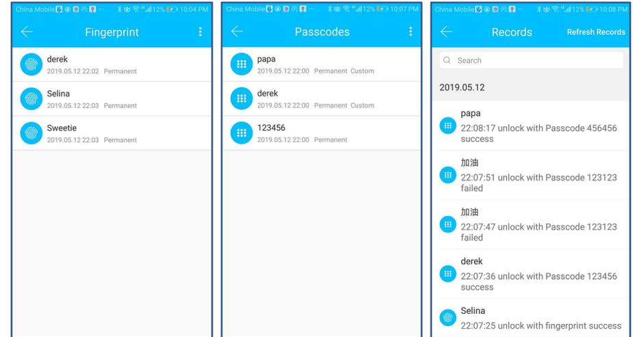
In the main interface of the TTLock App, select Passcodes, Fingerprints or IC Cards, and click on the upper right to add and manage fingerprints, passcodes and IC cards. You can add users for limited time or permanent access. The access records can be queried in the main interface.
